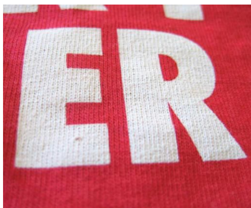
Discharge printing removes the original dye from the T-shirt and then adds a decoration that leaves no hand, as evidenced with this white discharge ink decoration from Forward Printing (circle 126 on Free Info Card).
